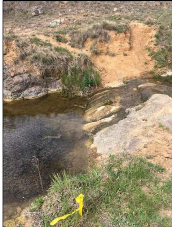
Upstream Marker Peg Positioned on left bank on high spot aligned with waterline of boulder step.
